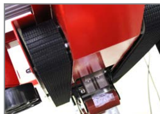
CINGHIE SUPERIORI MOTORIZZATE TWO TOP BELT CONTROLLED BY A MOTOR
